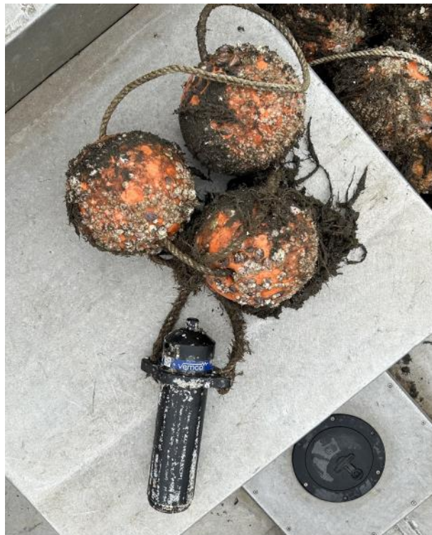
An acoustic receiver that was retrieved from the bottom of Long Island Sound. Fish transmitter information logged by the receiver is then downloaded, allowing researchers to analyze the date and time of fish locations and movements.
